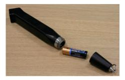
3. Insert battery back into the ProxiPen ensuring the positive (+) end is inserted into the main body of the ProxiPen.
